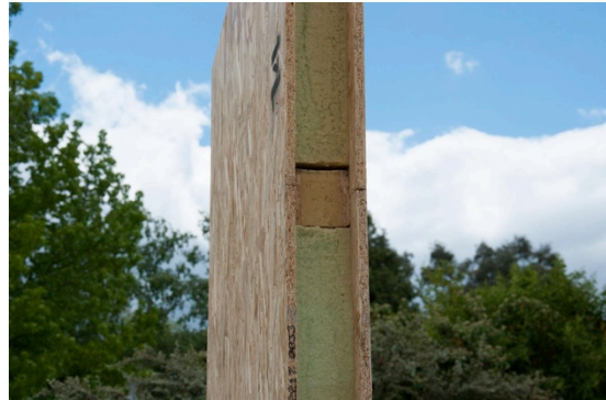
PIR wall insulation (90mm, U = 0.29 \text{ W/m}^2\text{K} )
